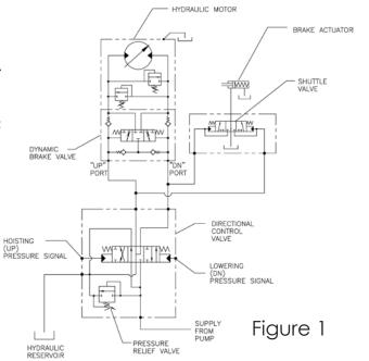
Seatrax cranes use **open loop** hydraulic systems. The hoist portion of this **hydraulic system** schematic is demonstrated in **Figure 1.** The system consists of the following major components:
