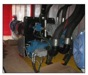
Dedicated hydraulic pumps are used for the primary crane functions. The hydraulic pumps are driven via a quad-pump drive, which is coupled to the electric motor by a flexible coupling.
