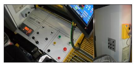
**Electro-hydraulic crane** standard cab control panel and electrical enclosures.
