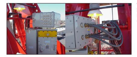
The collector ring assembly is located at the top of the kingpost/gantry. To the left is a collector ring for Zone 2.
