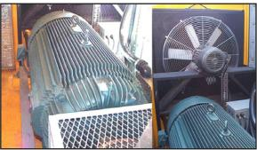
Electric motors are available for 60 Hz or 50 Hz applications. An auxiliary electric motor powers the fan for the hydraulic heat exchanger.
