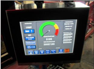
The Seatrax CCM14000 simplifies the monitoring of primary and auxiliary crane systems, including hydraulic systems, hoists and prime mover. It incorporates a hard wired network of boom angle and hoist load cell sensors that communicate with the display terminal.
