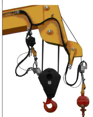
Hanging Weight Type Anti-Two Block with Boom Tip Mounted Valves
