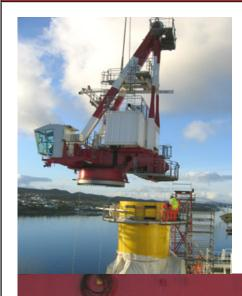
The revolving superstructure of a roller bearing type crane bolts on top of a roller bearing that is subjected to the full overturning moment from the weight of the load and the self-weight of the crane and boom.
