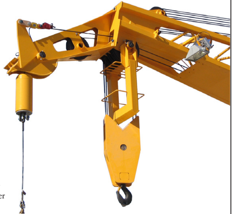
Mechanical Anti-Two-Block System Simple Seatrax arrangement for use on high use floating cranes.
