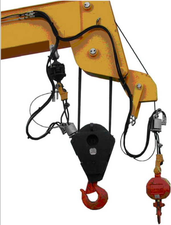
Mechanical Anti-Two-Block System Simple Seatrax arrangement for use on high use floating cranes.
