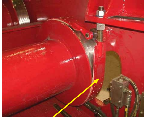
Seatrax Draw-Works-Type Band Brake Works DIRECTLY on the Drum
